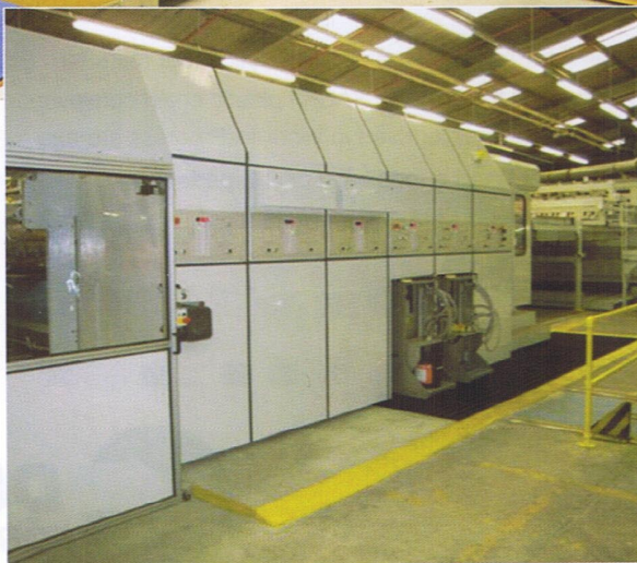
The BGM 16/45 Container Line is equipped with two flexo print units.
