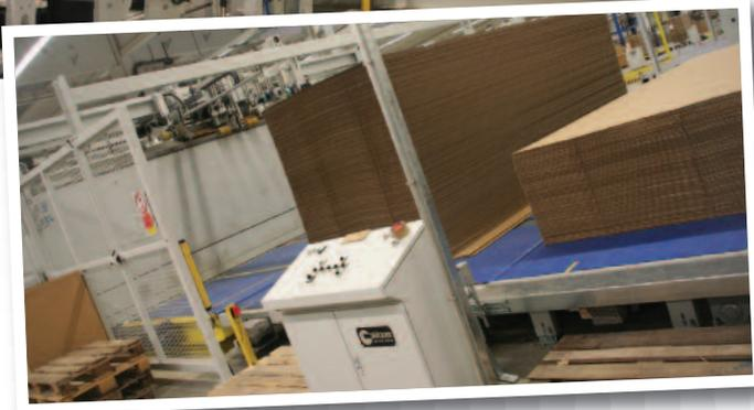
THE FOLDING SECTION FROM BAHMÜLLER IS THEIR LATEST SERVO DRIVEN, THREE BRIDGE DESIGN WHICH IS EQUIPPED WITH PATENTED STEP FOLDING BELTS. THESE ENSURE ACCURATE, SQUARE FOLDING AND GAP CONTROL, AND ELIMINATES MANY OF THE CAUSES OF FISHTAILING.
